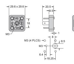
This DIN 43650 Form "A" / ISO 4400, EN175301-803:2000 male connector is specifically designed for mounting in sheet metal. It has an arc over insulating plastic ridge and includes a gasket and four mounting screws. The P10222 connector is designed to mate with Series 5000 or other DIN 43650 Form "A" / ISO 4400, EN175301-803: 2000 female connectors.
