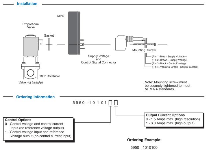
ISO molded 6 ft. cordset, control voltage and control current input, 1.5 amps max. output
