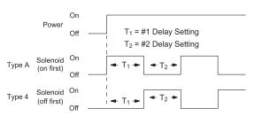
Solenoid cycles  $\Delta T_1$  OFF and  $\Delta T_2$  ON when power is applied. Reset occurs when power is removed. Timer is available in normally on (Type A) or normally off (Type 4) versions.
