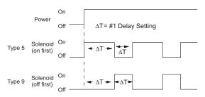
Solenoid cycles with equal ON and OFF times when power is applied. Reset occurs when power is removed. Timer is available in normally on (Type 5) or normally off (Type 9) versions.
