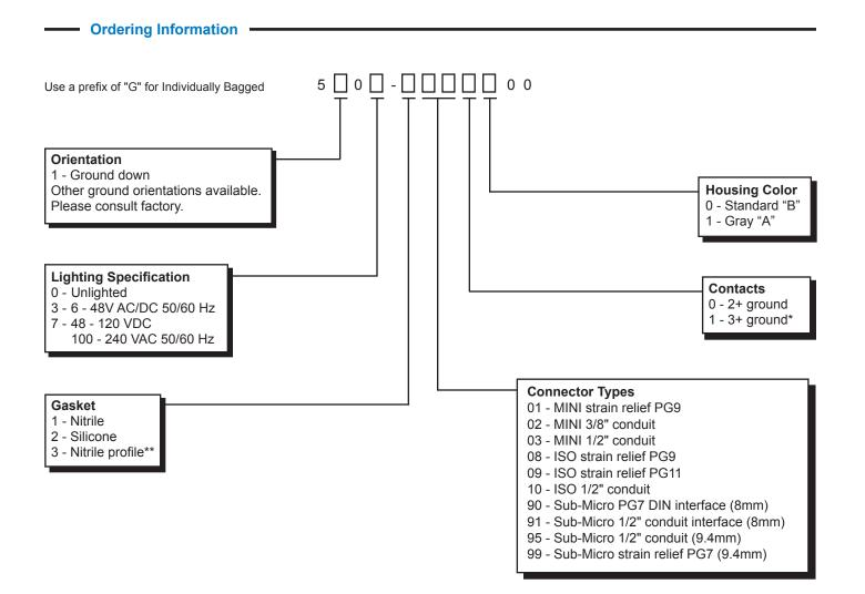
Each connector kit contains fastening hardware and gasket assembly.
